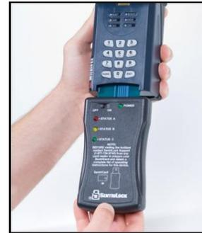
2. Slide the **Power** switch on the power paddle to the **ON** position. The green **POWER** light will illuminate.
