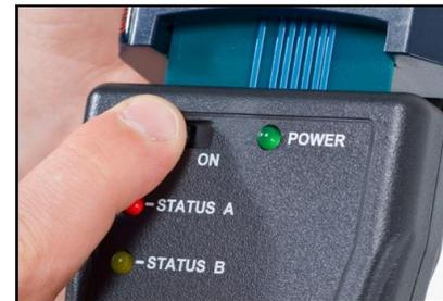
3. Once the power paddle is turned on, the red **Status A** light will illuminate for approximately one minute. During this time, the power paddle is charging the lockbox.
