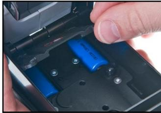
4. Remove the two CR123A batteries with a screwdriver (or a finger) and dispose of them properly.
