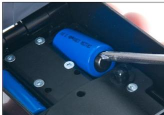
5. Using two, new CR123A batteries, install each battery into their battery cavity with the positive terminal going in first. The terminals are staggered, so the batteries will be facing different directions. Refer to the battery cover for proper battery terminal positions.
